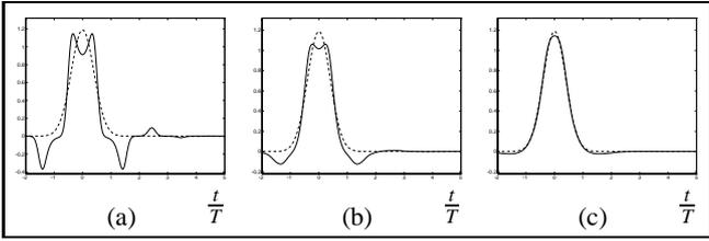
Figure 1: A Gaussian analysis window  $w(t)$  (dashed line) and its corresponding optimum synthesis window  $g_{opt}(t)$  (solid line) for different values of oversampling: (a)  $\alpha = \beta = \sqrt{6/7}$ , (b)  $\alpha = \beta = \sqrt{2/3}$ , and (c)  $\alpha = \beta = \sqrt{2/5}$ .
