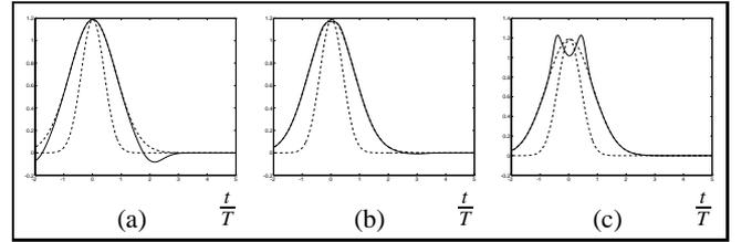
Figure 3: A Gaussian analysis window  $w(t)$  (dashed line), a required Gaussian-shaped function  $f(t)$  with double width (dashed line), and the corresponding optimum synthesis window  $g_f(t)$  (solid line) in the case of oversampling by a factor 4, for different values of  $\alpha$  and  $\beta$ : (a)  $\alpha = \beta = 1/2$ , (b)  $\alpha = \sqrt{2}/2$ ,  $\beta = \sqrt{2}/4$ , and (c)  $\alpha = 1$ ,  $\beta = 1/4$ .
