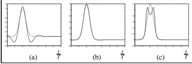
Figure 2: A Gaussian analysis window  $w(t)$  (dashed line) and its corresponding optimum synthesis window  $g_{opt}(t)$  (solid line) in the case of oversampling by a factor 3, for different values of  $\alpha$  and  $\beta$ : (a)  $\alpha = 1/3$ ,  $\beta = 1$ , (b)  $\alpha = \beta = \sqrt{1/3}$ , and (c)  $\alpha = 1$ ,  $\beta = 1/3$ .
