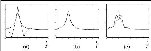
Figure 4: An exponential analysis window  $w(t)$  (dashed line) and its corresponding optimum synthesis window  $g_{opt}(t)$  (solid line) in the case of oversampling by a factor 9, for different values of  $\alpha$  and  $\beta$ : (a)  $\alpha = 1/9$ ,  $\beta = 1$ , (b)  $\alpha = \beta = 1/3$ , and (c)  $\alpha = 1$ ,  $\beta = 1/9$ .
